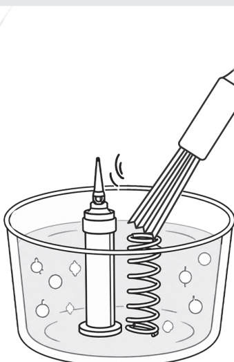
❷ Clean the Needle and Spring
