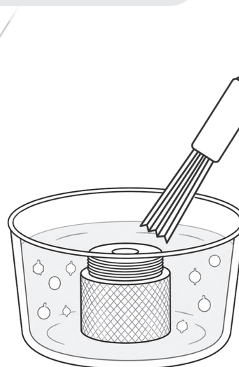
❸ Clean the Paint Control Cap
