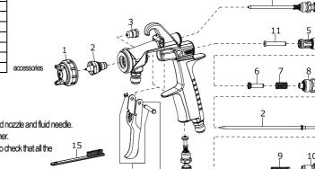
Marked parts are wearable parts.
